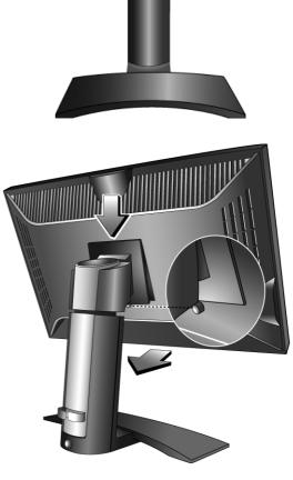
3. Fully extend and tilt the monitor to rotate it.
